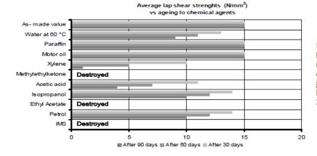
If not specified, the tests have been conducted at 20°C after immersion for 30, 60 and 90 days at 20°C on steel to steel joints which have been hardened for 48 hours at 20°C.
