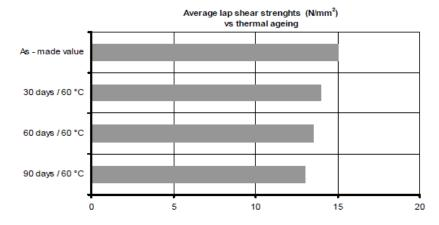
The tests have been conducted at 20°C on steel to steel joints, which have been aged at 60°C.
